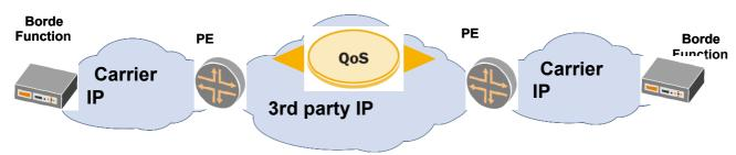
Figure 66 – Layer 3 Private-oriented Interconnection Configuration
