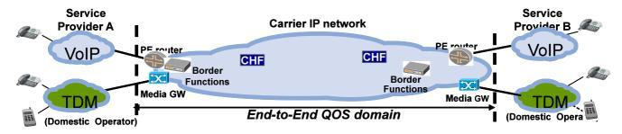
Figure 12 –QoS Measurement for single network domain
