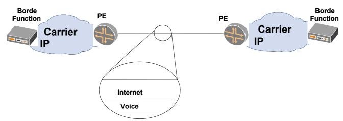
Figure 77 - Layer 1 / 2 Public-oriented Direct Interconnection Configuration
