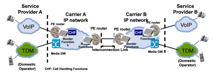
Figure 11 - Reference Configuration for QoS Measurement
