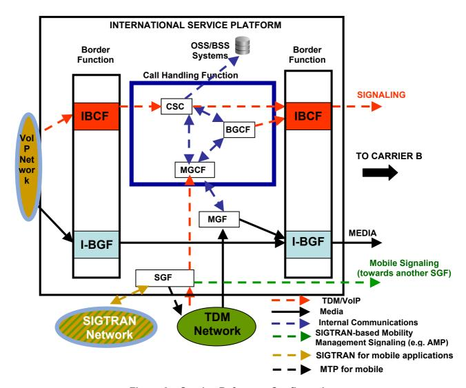
Figure 2 - Service Reference Configuration
