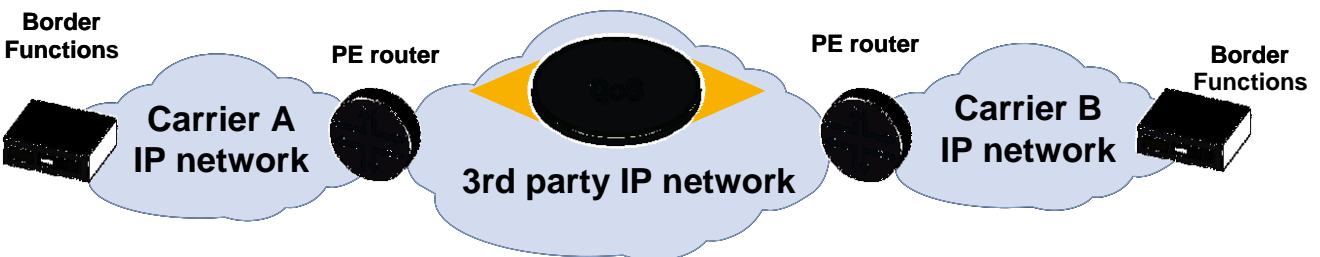
Figure 66 – Layer 3 Private-oriented Interconnection Configuration
