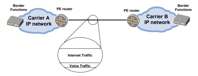
Alt. 2) Non direct interconnection via Public Internet (see figure below): the VoIP traffic passes through Public Internet i.e. through a third (or multiple) Internet Transit providers. The IP addresses of the PE routers as well as of the Border functions shall be public and they shall be announced over the Public Internet.
