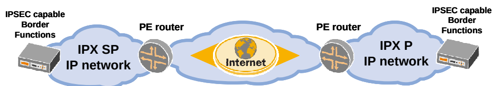
Figure 8 — Internet IPSEC SP/P Interconnection Configuration
