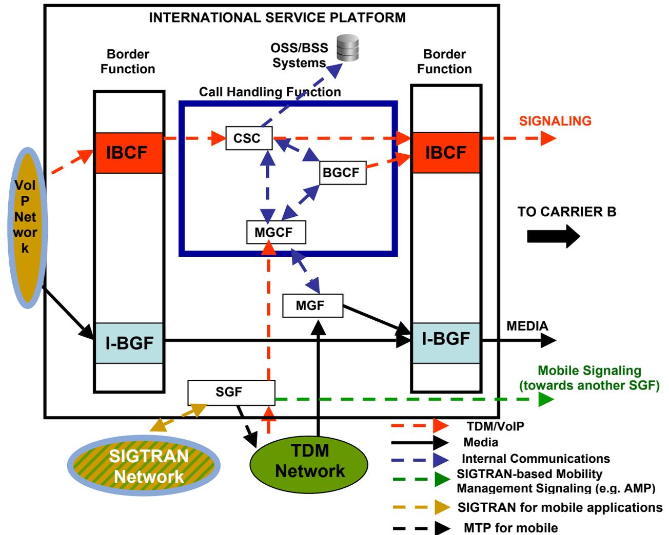
**Figure 2 – Service Reference Configuration**
