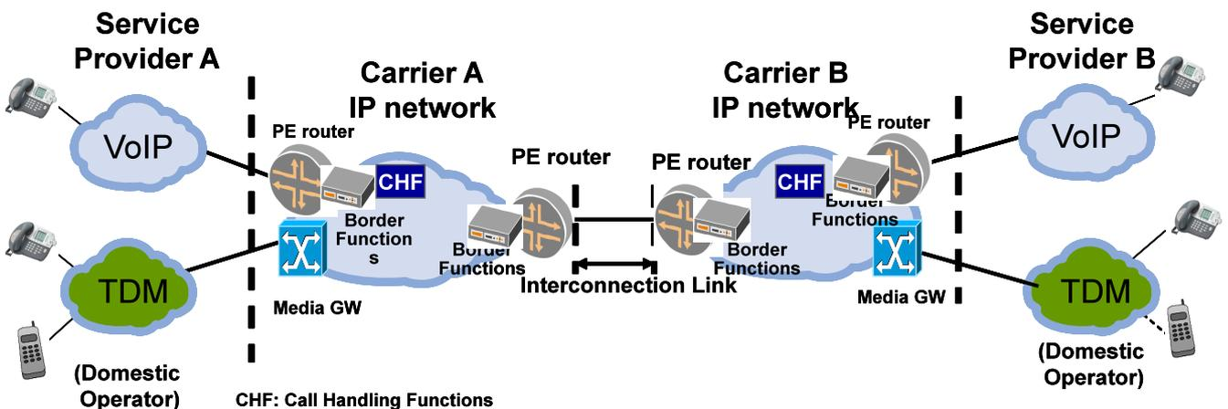
**Figure 11 – Reference Configuration for QoS Measurement**
