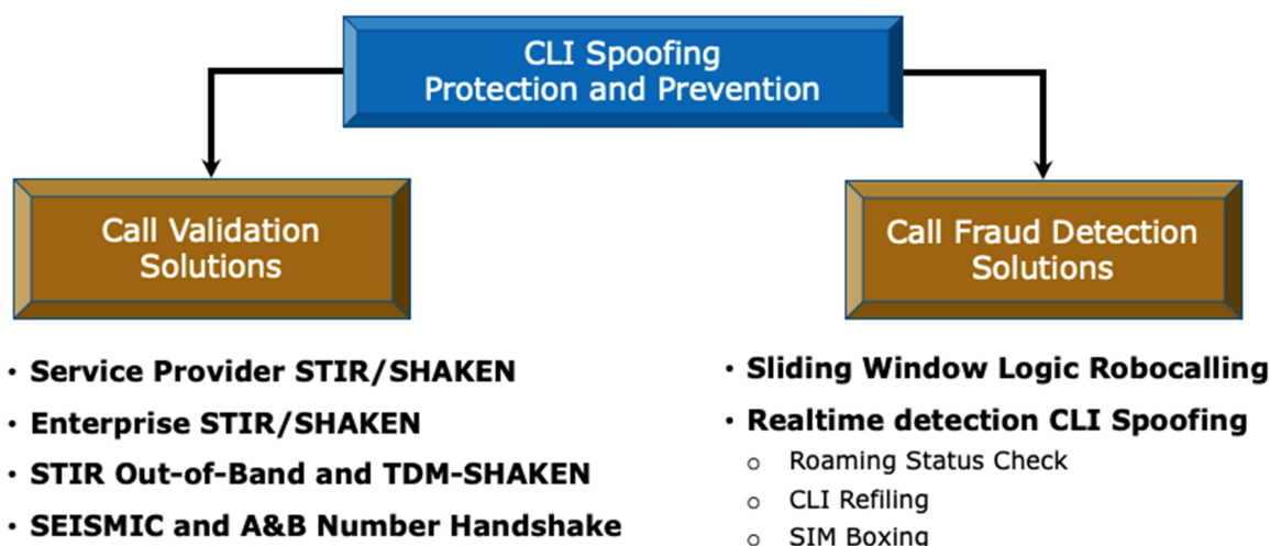
Figure 2 – Overview of Protection and Prevention Solutions for CLI Spoofing
