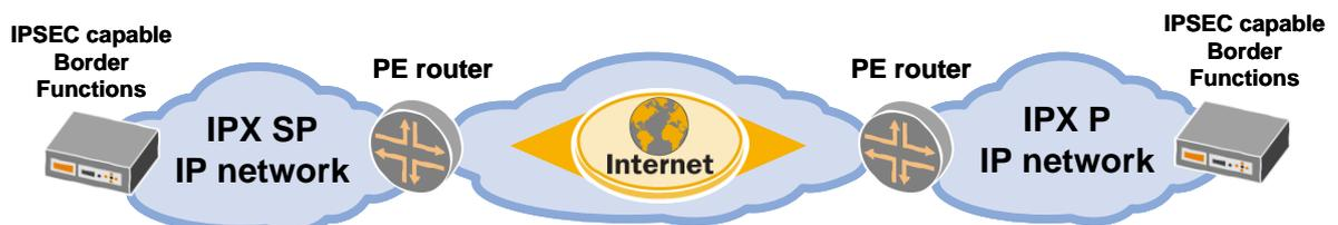
Figure 8 — Internet IPSEC SP/P Interconnection Configuration
